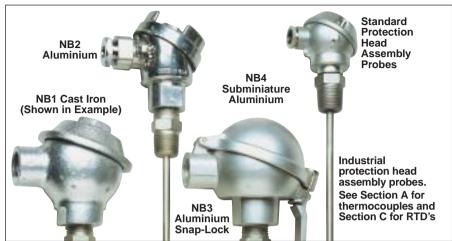
The ½" BSPT mounting thread allows 6mm (or ½) OD industrial protection head assemblies to be put directly into OMEGA® thermowells whose bore is 6.6mm without having to use any additional hardware. In this case, the probe length must be the same as the element (stem) length of the desired thermowell.
