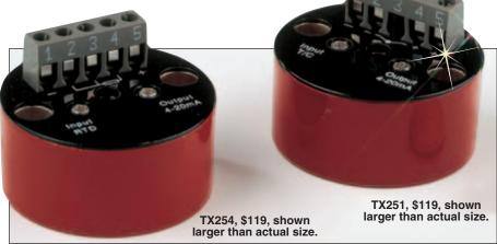
The TX254 transmitter is provided with excellent lead resistance compensation and Pt-100 linearization conforming to BS1904 and DIN 43760 characteristics (a = 0.00385).The transmitter calibration is set by 6 dip-switches located behind the top cover.
